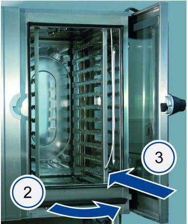
The illustration shows a stainless steel combi steamer with its door open. A blue arrow labeled '2' points to the door handle, indicating the opening action. A second blue arrow labeled '3' points to the door's edge, indicating it should be slid back along the side of the unit. The interior of the steamer is visible, showing several metal trays. |
